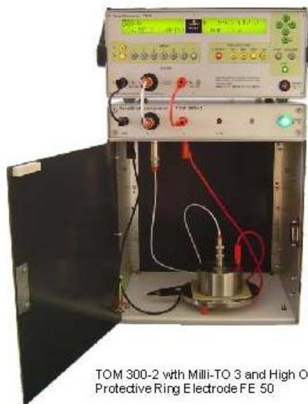
TOM 300-2 with Milli-TO 3 and High Ohm Protective Ring Electrode FE 50
